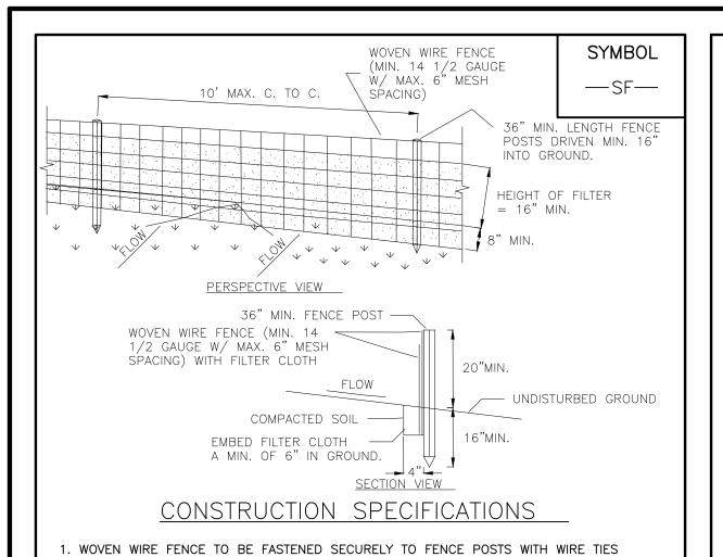
OR STAPLES. POSTS SHALL BE STEEL EITHER "T" OR "U" TYPE OR HARDWOOD. 2. FILTER CLOTH TO BE TO BE FASTENED SECURELY TO WOVEN WIRE FENCE WITH TIES SPACED EVERY 24" AT TOP AND MID SECTION. FENCE SHALL BE WOVEN WIRE, 12 1/2 GAUGE, 6" MAXIMUM MESH OPENING
