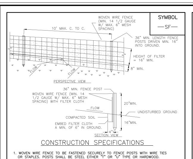
2. FILTER CLOTH TO BE TO BE FASTENED SECURELY TO WOVEN WIRE FENCE WITH TIES SPACED EVERY 24" AT TOP AND MID SECTION. FENCE SHALL BE WOVEN WIRE, 12 1/2 GAUGE, 6" MAXIMUM MESH OPENING 3. WHEN TWO SECTIONS OF FILTER CLOTH ADJOIN EACH OTHER THEY SHALL BE OVER-LAPPED BY SIX INCHES AND FOLDED. FILTER CLOTH SHALL BE EITHER FILTER X, MIRAFI 100X, STABILINKA T140N, OR APPROVED EQUIVALENT.
