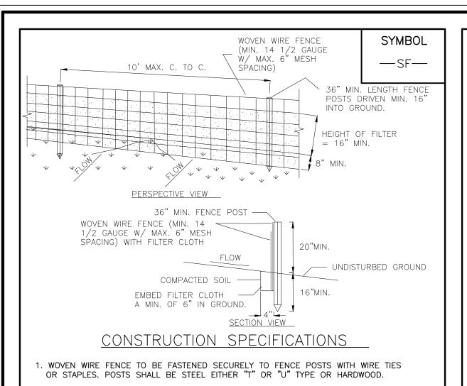
2. FILTER CLOTH TO BE TO BE FASTENED SECURELY TO WOVEN WIRE
